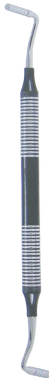
786-1586 Tamper Length 170mm, for bone material double ended, diameter 3.2 mm (2-4-6-8-10) and diameter 2.5mm (2-4-6-8-10)
